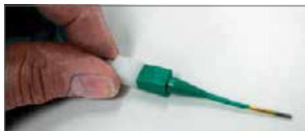
Plastic tool with contact in proper position.
