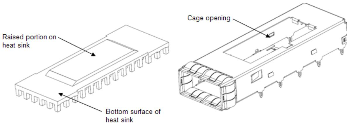
**FIGURE 6: Heat Sink and Cage Features**
