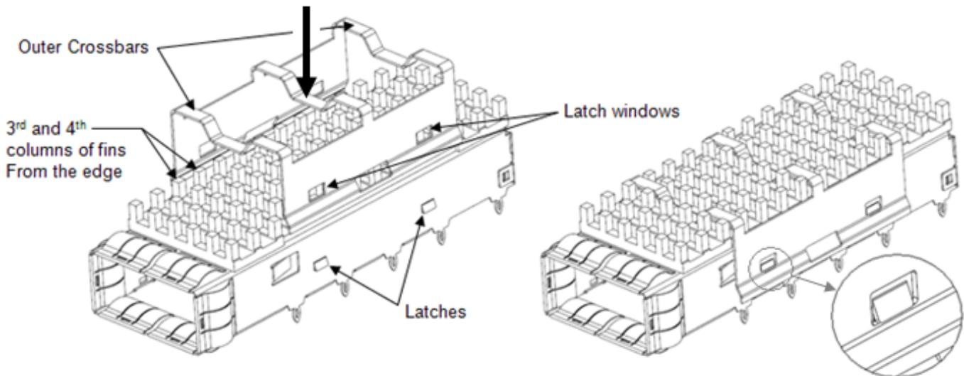
**FIGURE 7: Heat Sink Clip Assembly**
