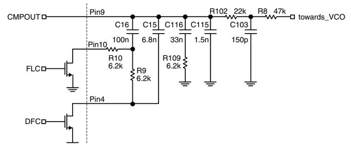
**Figure 7. Dual-Loop Filters**
