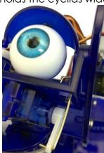
4. Tilt the eyebox up fix the arm onto the motor using screw B
