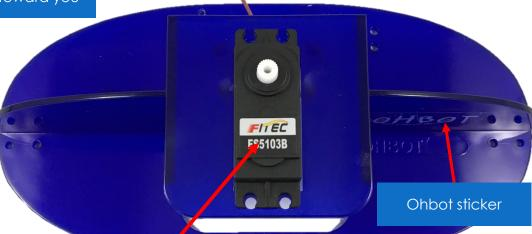
2. Thread the motor's cable through the big hole on the top of the base then put the motor in so that the writing on the label is the right way up.
