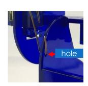
5. Find **Motor 4**. Push the arm onto the motor so it holds Ohbot's head **upright**.
