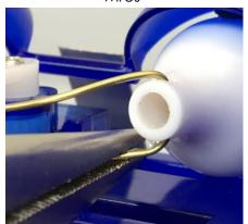
6. Fix the arm onto the motor using screw B
