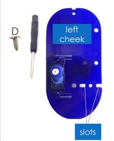
1. Locate the lugs of the jaw in the slots on the cheek
