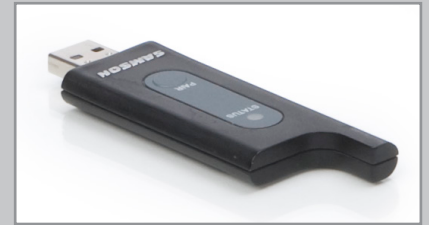
Wireless receiver built into a USB stick
