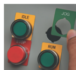
Control Panel Labels
