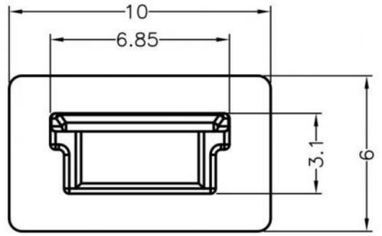
All measurement does not include gate which raises under 1.2mm.
