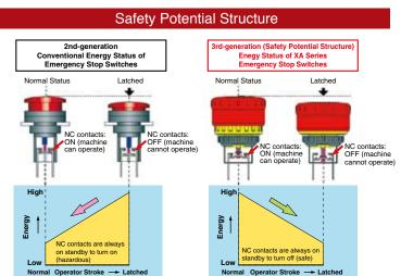
With XA emergency stop switches, the potential energy level of the latched status is lower than that of normal status. In the event the switch is damaged due to excessive shocks, the NC contacts will turn off, thus stopping the machine (patented).
