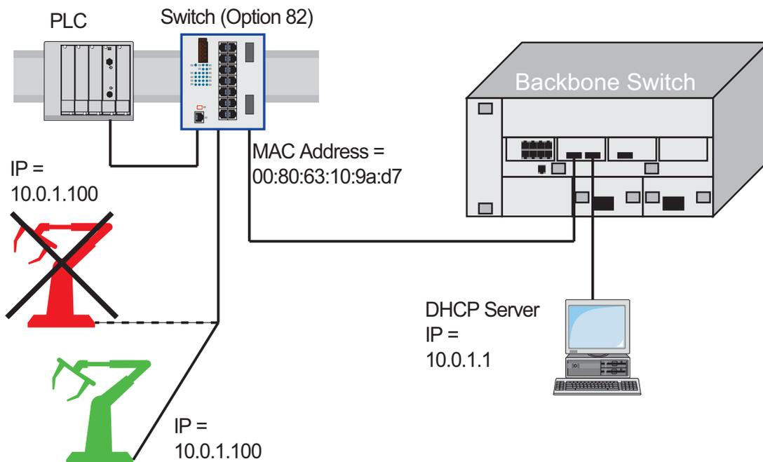
Figure 12: Application example of using Option 82
