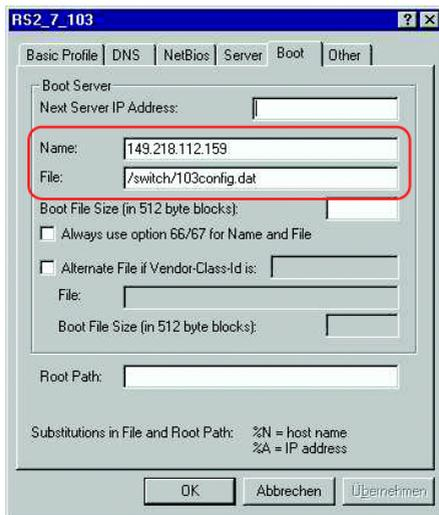
Figure 51: Configuration file on the tftp server
