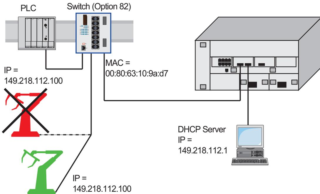
Figure 62: Application example of using Option 82
