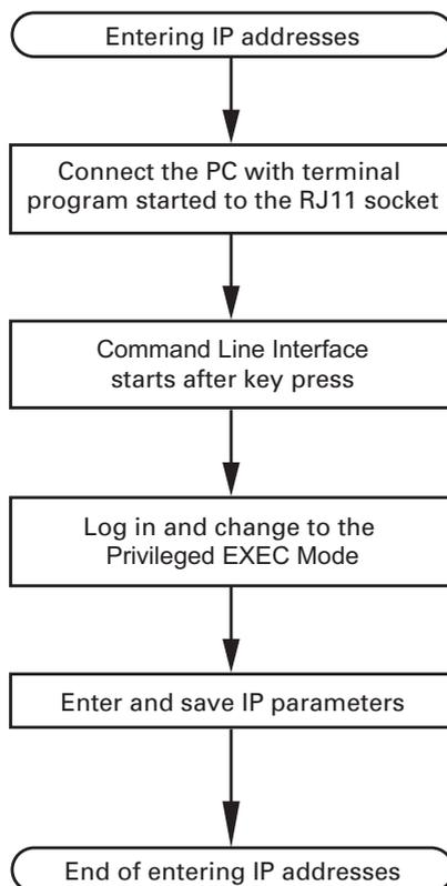
Figure 8: Flow chart for entering IP addresses
