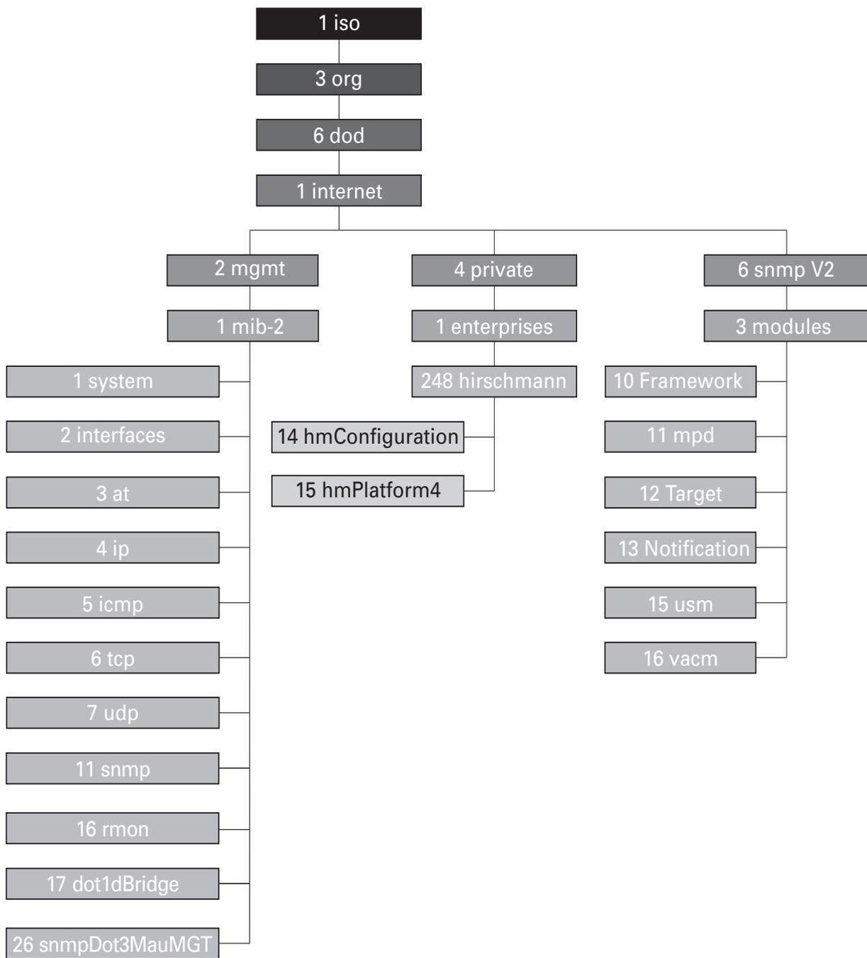
Figure 64: Tree structure of the Hirschmann MIB
