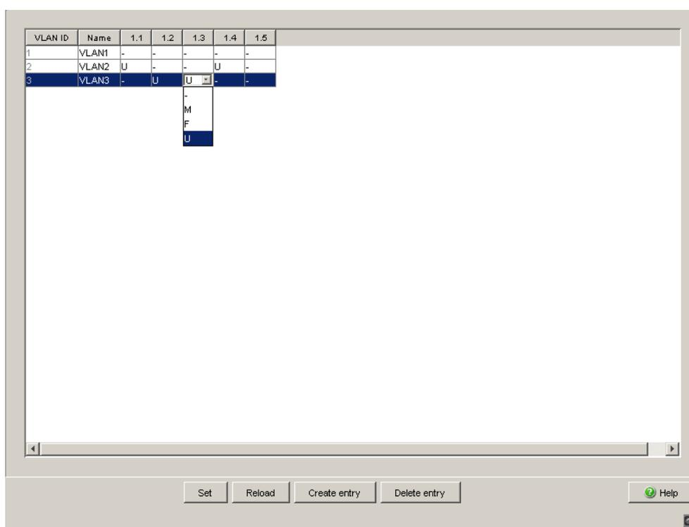
Figure 34: Defining the VLAN membership of the ports.
