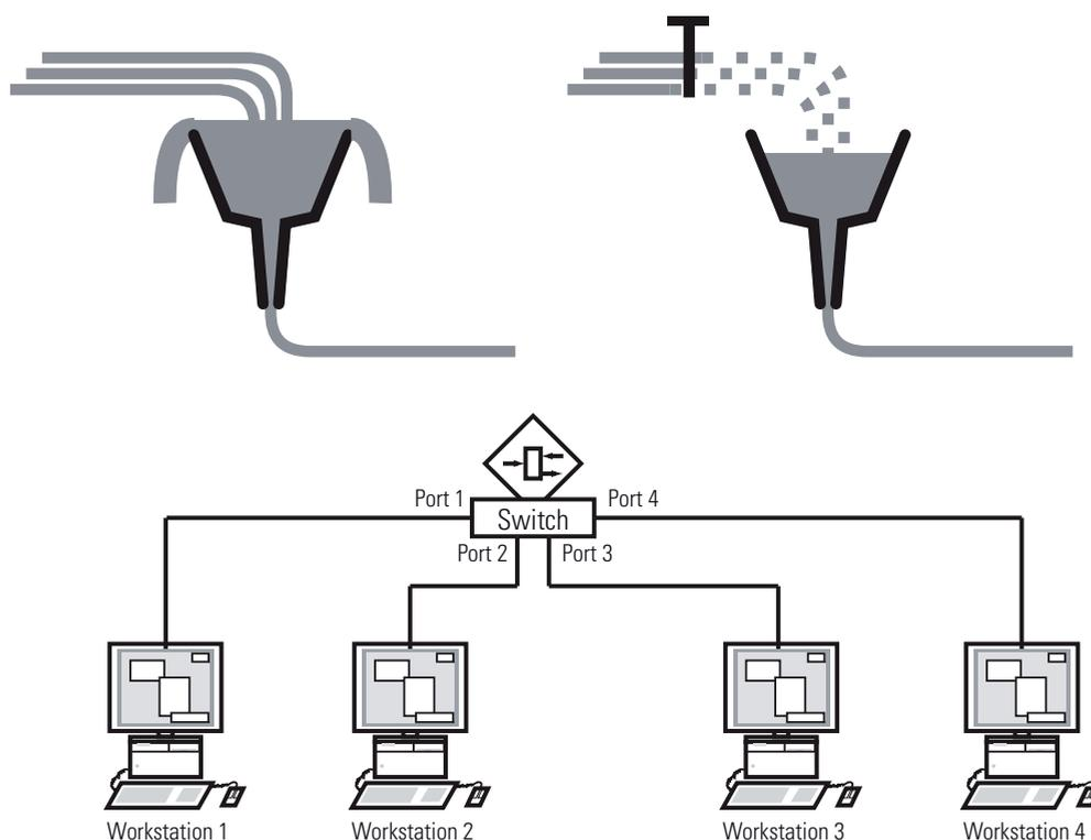
Figure 31: Example of flow control
