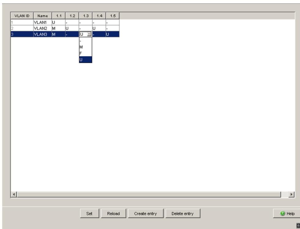
Figure 38: Defining the VLAN membership of the ports.
