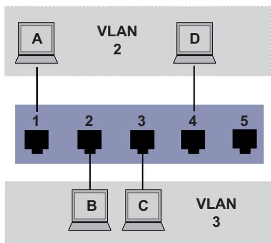
Figure 32: Example of a simple port-based VLAN
