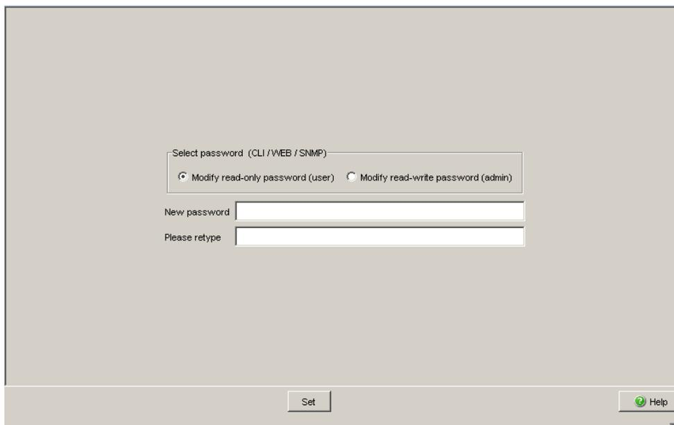
Figure 18: Password/SNMP Access dialog
