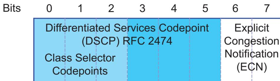
Figure 30: Differentiated Services field in the IP header
