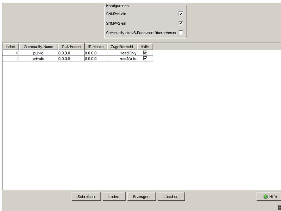
The screenshot shows a configuration dialog for SNMP access. At the top, there is a 'Konfiguration' section with three checkboxes: 'SNMPv1 ein' (checked), 'SNMPv2 ein' (checked), and 'Community als v3-Passwort übernehmen' (unchecked). Below this is a table with the following data:
