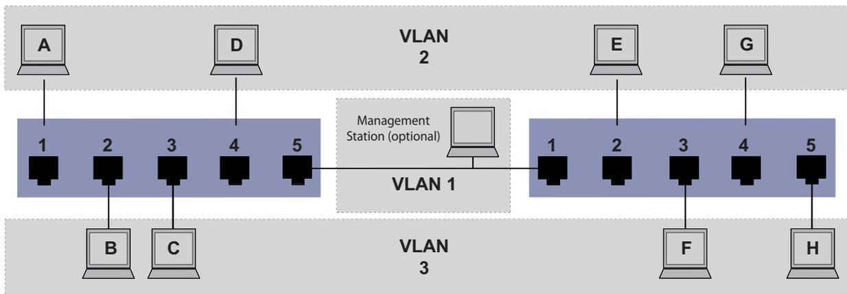
Figure 36: Example of a more complex VLAN configuration
