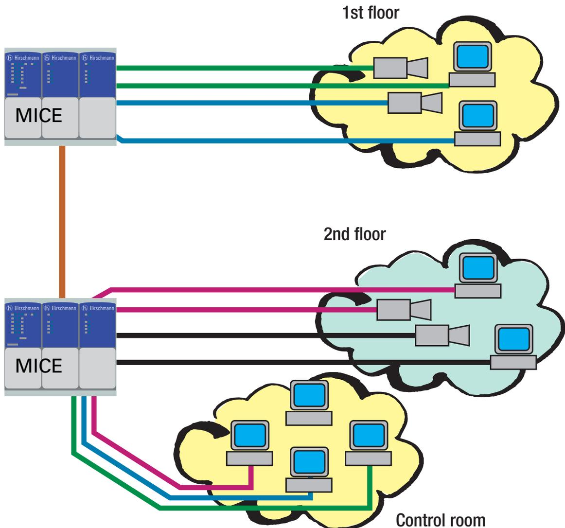
Figure 25: Example: Video surveillance in machine rooms
