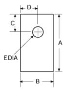
Aavid Aluminum Oxide Ceramic for a TO-220 device. Surface flatness is 0.05mm (0.002 TIR).
