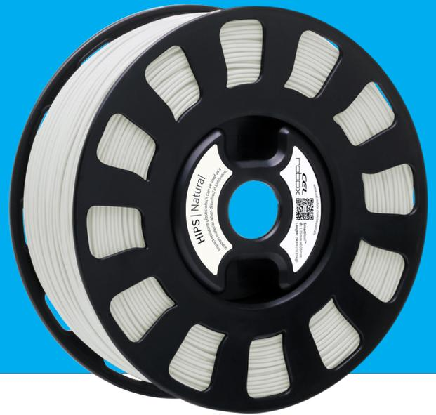
Robox® HIPS is a material with a unique matte finish and structure that reduces the visibility of minor flaws, making it ideally suited for producing eye-catching prototypes. HIPS can also be used with ABS as a breakaway support material or a soluble support material for PETG parts when dissolved with d-Limonene.
