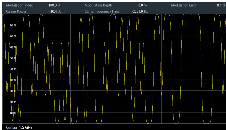
Figure 13-4: Modulation depth of a 2ASK signal
