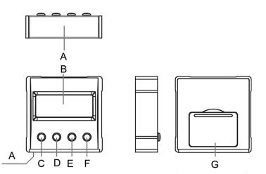
A ..... Stainless steel sheet-Measuring faces,Securely attaches gauge to any metal surface.
