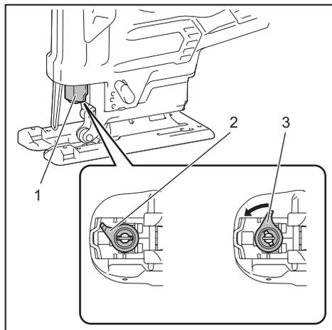
▶ 1. Jig saw blade holder 2. Released position
