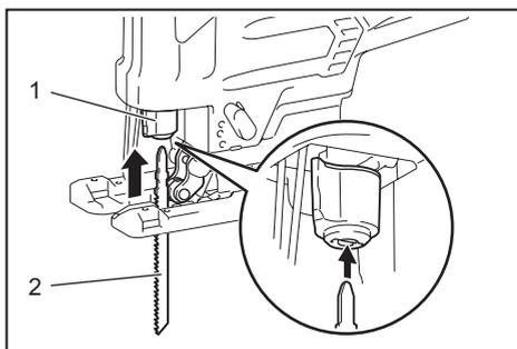
▶ 1. Jig saw blade holder 2. Jig saw blade
