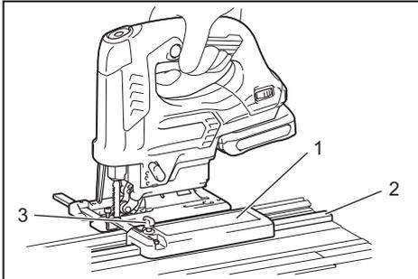
► 1. Guide rail adapter 2. Guide rail 3. Screw
