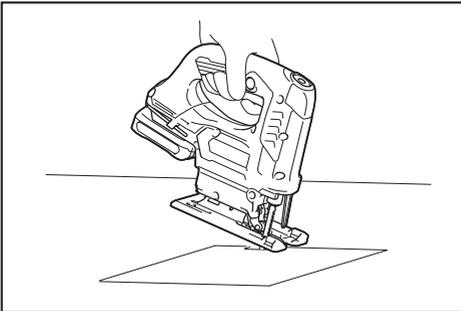
You need not bore a starting hole or make a lead-in cut if you carefully do as follows.
