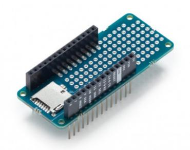
The **Arduino MKR SD Proto Shield** allows you to easily connect an SD card to your MKR form factor board. Use it to enhance the IoT features of your MKR1000, as well as store data coming from the web or sensors read by your board!
