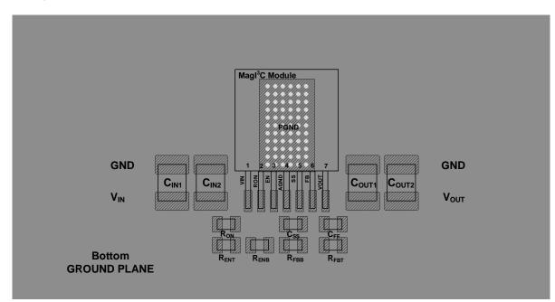
Place a dedicated solid GND copper area beneath the MagI<sup>3</sup>C Power Module.
