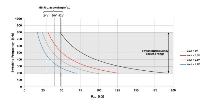
As stated above, the off-time is also limited to a minimum value of 260 ns, which limits the maximum duty cycle. Larger  $R_{ON}$  (lower  $F_{SW}$ ) should be selected in any application requiring large duty ratio.
