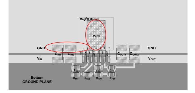
The negative terminal of C<sub>IN1</sub> and C<sub>IN2</sub> needs to be very close to the PGND pad of the power module.
