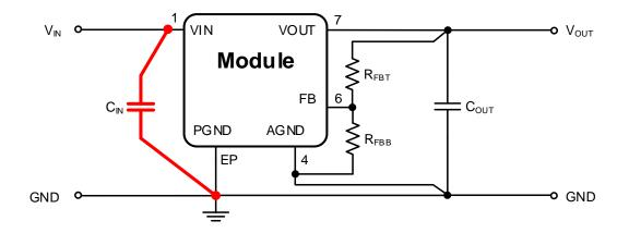
Based on those considerations, the path of the input capacitor  $C_{IN}$  is the most critical one to generate high frequency noise on  $V_{IN}$ . Therefore place  $C_{IN}$  as close as possible to the Magl<sup>3</sup>C power module  $V_{IN}$  and PGND exposed pad EP. This will minimize the high di/dt area and reduce radiated EMI. Additionally, grounding for both the input and output capacitor should consist of a localized top side plane that connects to the PGND exposed pad.
