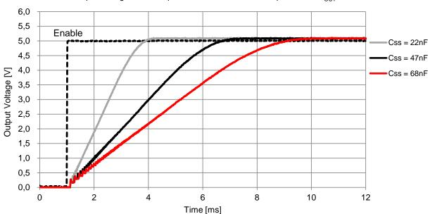
Output Voltage at Start Up with Different Soft-Start Capacitors at  $V_{OUT} = 5V$
