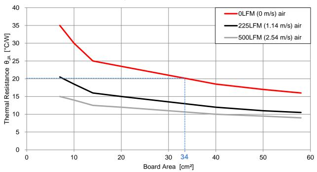
Package Thermal Resistance  $\theta_{JA}$  - 4 Layer PCB with 35µm copper and 36 thermal vias
