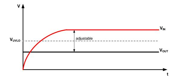
Magl<sup>3</sup>C Power Module VDRM – Variable Step Down Regulator Module
