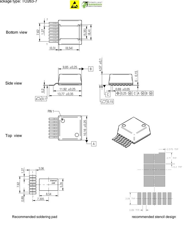
Magl<sup>3</sup>C Power Module VDRM – Variable Step Down Regulator Module
