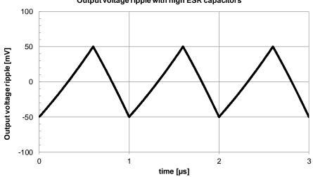
Output voltage ripple with high ESR capacitors
