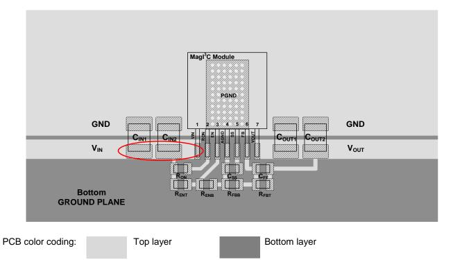
The positive terminal of  $C_{IN1}$  and  $C_{IN2}$  need to be very close to the VIN pin of the power module.
