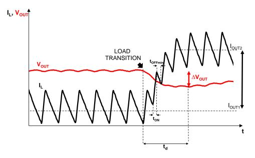
The selection of the C<sub>OUT</sub> is related to the t<sub>d</sub> as well as to the current step  $\Delta I_{OUT}$  and the max allowed voltage drop  $\Delta V_{OUT}$ , as shown by the following equation:
