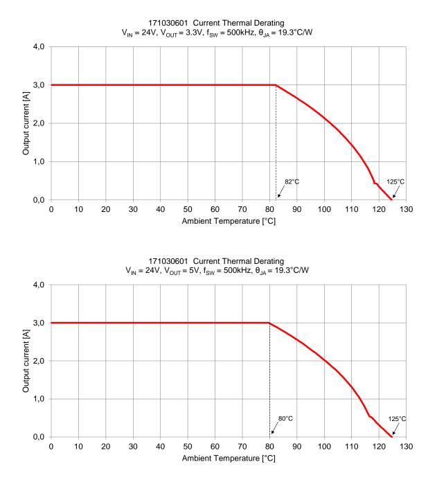
The ambient temperature and the power limits of the derating curve represent the operation at the max junction temperature specified in the "<u>Operating Conditions</u>" section on page 4.
