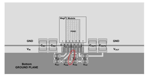
The ground connections for the soft-start capacitor (C<sub>SS</sub>), the output voltage lower resistor divider (R<sub>FBB</sub>) and enable components (when used) should be routed to the AGND pin of the device. If not properly handled, poor grounding can result in degraded load regulation or erratic output voltage ripple behavior. Place C<sub>SS</sub>, R<sub>FBT</sub> and R<sub>FBB</sub> close to their respective pins.
