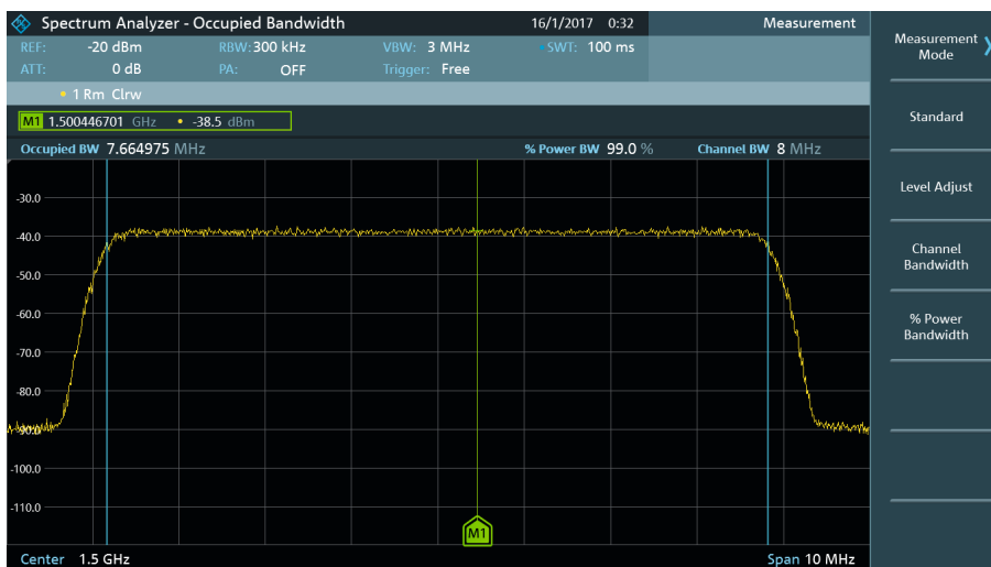
R&S®FPC-K55: occupied bandwidth.
