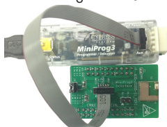
Fig 3: Programming/Debugging with MiniProg3
