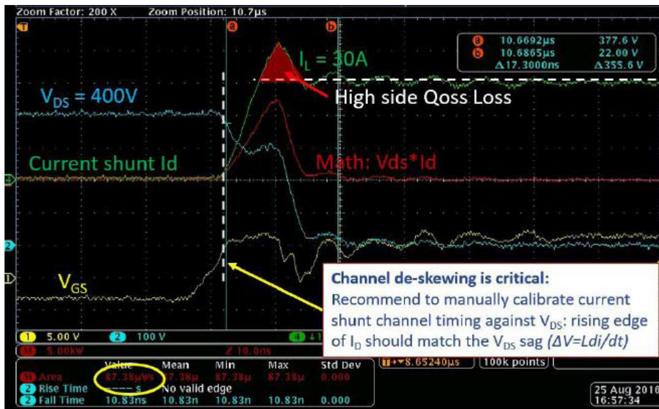
Figure 10: Turn-On Switching Loss Measurement
