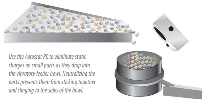
Use the Aerostat PC to eliminate static charges on small parts as they drop into the vibratory feeder bowl. Neutralizing the parts prevents them from sticking together and clinging to the sides of the bowl.
