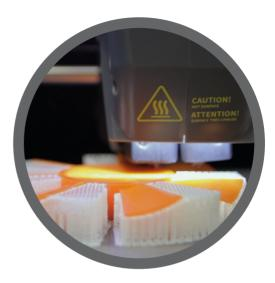
Robox needle valve nozzle control technology for reduced print times.
