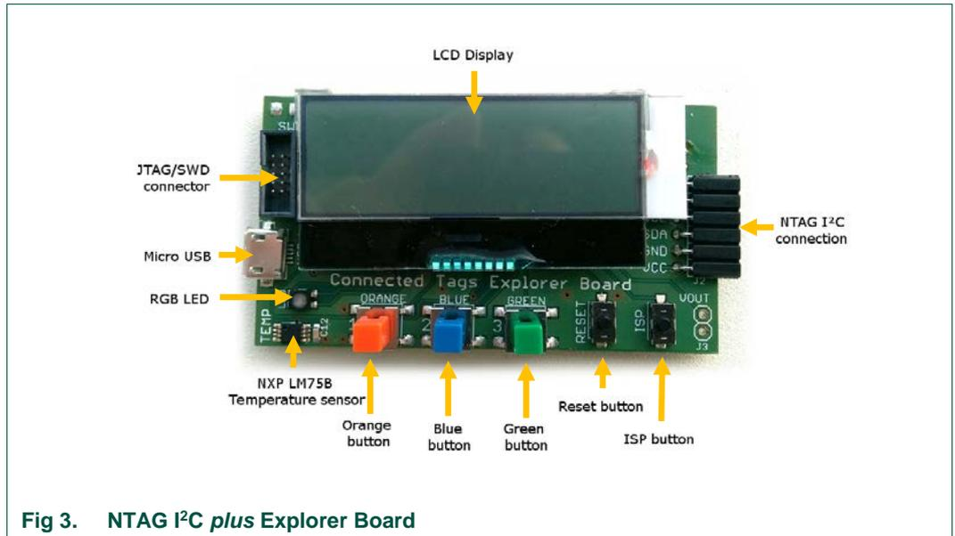
Fig 3. NTAG I<sup>2</sup>C plus Explorer Board
