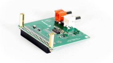
The longer spacers will be mounted on the side with the 40-pin connector.
