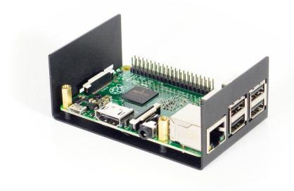
You have to mount the shorter standoffs on the side with the power/HDMI/audio connectors, not on the side with the 40-pin connector.
