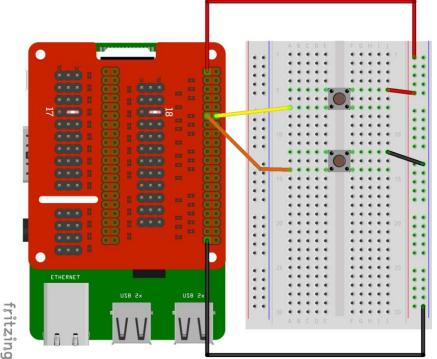
The button connected to the 3v3 line on the breadboard should be connected to GPIO18 / PIN12. We need to pull GPIO18 LOW, to do this, simply place a jumper between the middle pin and the top pin where the bank of pins are labelled 18. Notice the letter "d" and "u" on the edge of the PCB, this indicates which "way" the pins are being pulled, u = UP, d = DOWN.
