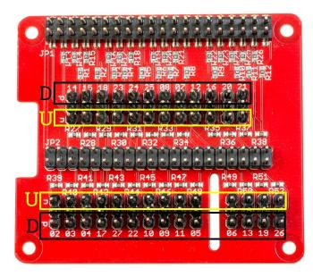
Once that's all wired up, you can copy the code below, and execute it. The code will show the initial states of our inputs, which should be 1 for the button pulled up and 0 for the button pulled down. When a button is pressed these values should change. So the button connected to the 3v3 line should change to 1, and the button connected to the ground line should change to 0.
