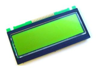
A high quality 16x2 char STN LCD module. It uses the industry standard LCD interface, 16 way 1.27mm pitch. The module measures 59mm x 29.5mm, display area is 64mm x 15mm, two mounting centres are 50mm apart. Overall thickness including bezel is 3.8mm (4.8mm for chip locations). Supplied with protective screen layer and a 15-way connector (rightmost pad of LCD is not used).
