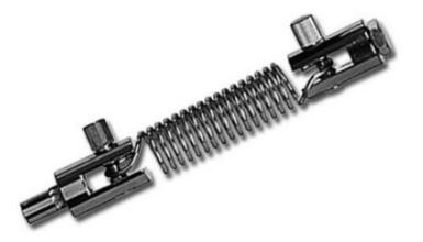
NIDEC-SHIMPO's Clevis Grip easily attach and secure odd shaped parts, punched samples or tension springs. Concave shape of pins assures centering under load. Throat clearance with pin is 0.5" (12.7 mm) and can easily accept samples up to 0.375" (9.65 mm) wide.
