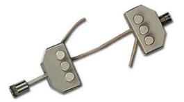
NIDEC-SHIMPO's Cord and Twine Grip attachments contain a figure 8 wrap that assures a center break. These grips feature non-locking pins which permit quick installation and release.
