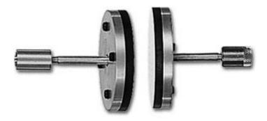
SHIMPO's Adhesive Test Plate attachments with hardened tool steel, detachable face-plates can test samples up to 3" (76.20 mm) in diameter. Ball socket mounting screws in both grips assure parallelism and perpendicularity to force when load is applied.
