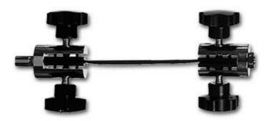
SHIMPO's Heavy-duty Tensile Grip attachments with manually tightened jaw faces can accept samples 1.25" (31.75 mm) wide and 0.25" (6.35 mm) thick. Contact faces are serrated hardened tool steel.
