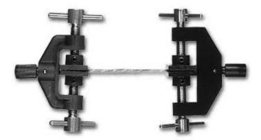
NIDEC-SHIMPO's Flat Chuck Tensile Grip attachments possess a 0.79" (20 mm) square, serrated gripping face that can accept samples up to 0.75" (19 mm) thick.
