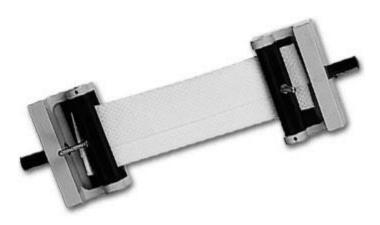
NIDEC-SHIMPO's Fabric Grip attachments are eccentrically mounted and contain serrated roller grips that allow for self-tightening of specimens up to 3" (76.20 mm) wide and 0.25" (6.4 mm) thick.
