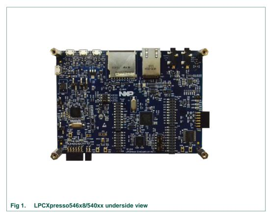
This document describes the hardware of the LPCXpresso546x8/540xx boards, plus information on the CAN-FD shield supplied in the OM13094 kit (this shield board is also available as a standalone product, order code OM13099.) This shield board can be used with any of the LPCXpresso boards described, but the LPCXpresso54608 does not support CAN-FD.
