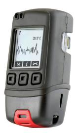
This stand-alone data logger measures and stores over 250,000 temperature readings over a -30 to +80°C (-22 to +176°F) range at a resolution of 0.1°C
