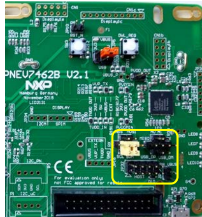
Fig 19. Host Interface selection - I2C mode
