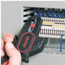
Stripping in confined areas
