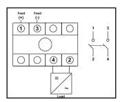
Note: 2 strings can be connected to one switch (2 poles per string) as long as each string does not exceed 500V and the current does not exceed the rating of the switch. However, for maintenance and isolation purposes, it is recommended that 1 isolator is used per string
