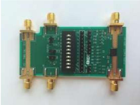
The F1956EVBI is a fully populated evaluation board which allows the customer to easily evaluate the F1956 digital step attenuator. Attenuation may be set using either the F1956's parallel control input or its serial control input. A dip switch on the evaluation board allows one to set the attenuation state without off-board connections to the control inputs.
