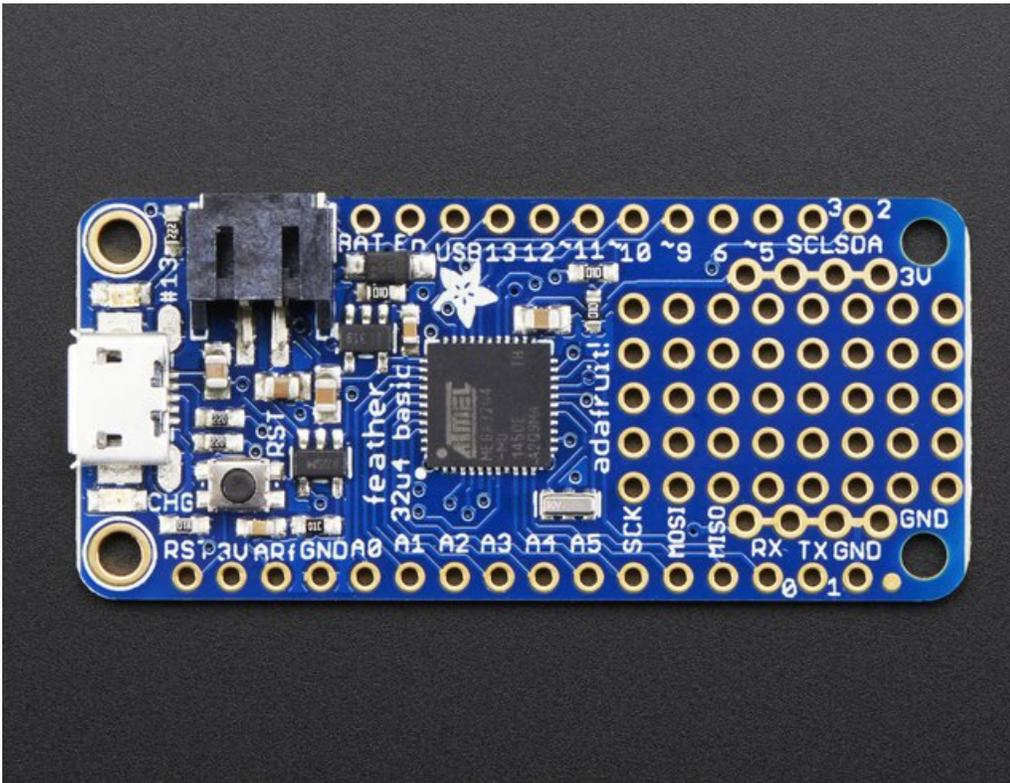
At the Feather 32u4's heart is an ATmega32u4 clocked at 8 MHz and at 3.3V logic, a chip setup we've had tons of experience with as [it's the same as the Flora](#). This chip has 32K of flash and 2K of RAM, with built-in USB so not only does it have a USB-to-Serial program & debug capability built in with no need for an FTDI-like chip, it can also act like a mouse, keyboard, USB MIDI device, etc.
