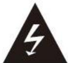
This symbol is intended to alert the user to the presence of “dangerous” voltage within the product’s enclosure that may be of sufficient magnitude to constitute a risk of Electric shock. Users should exhibit extra safety when this symbol appears in this instruction manual and follow all precautions as they are stated.
