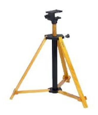
The Tektronix EMI-TRIPOD is the Com-Power AT-812 antenna tripod that supports the ABF-900 and ALC-100 antennas for EMC testing. The tripod is made of non reflective nylon and wood material. The antenna height can be easily adjusted by moving the center slotted rod up or down. The tripod is designed to be portable so that the antenna can be placed at the appropriate location for testing. The tripod legs can be folded for easy transport and storage.
