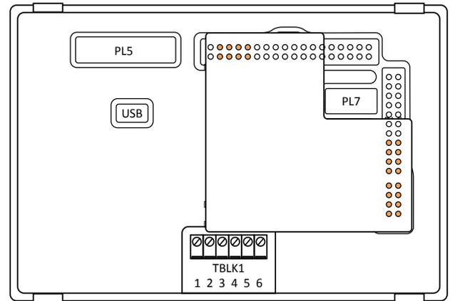
The diagram (above-right) indicates the pins on the SGD 43-A that the S43-TP should be connected to.
