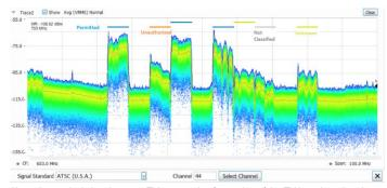
Above is a typical signal survey. This survey is of a portion of the TV broadcast band, and 7 regions have been declared as either Permitted, Unknown, or Unauthorized, as indicated by the color bars for each region.
