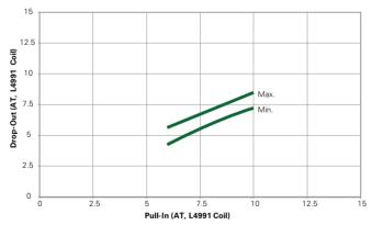
Note: The chart represents the range of Drop-Out, minimum to maximum for a given Pull-In value.
