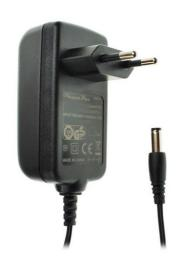
This switch mode power supply is rated to 12W maximum, providing a regulated 24vdc output at up to 0.5A with no minimum load. The unit meets Level VI COC Tier 2 efficiency standards. This power supply carries full safety approvals. Short circuit and over current protection is integral.
