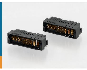
TE Connectivity's MULTI-BEAM XLE connectors are the latest addition to the MULTI-BEAM XL power connector product family. MULTI-BEAM XLE connectors feature a new 3-beam contact, made from a thicker (higher) conductivity material than the original single-beam or 4-beam designs. The new 3-beam design allows for a greater angular mis-alignment between mating connectors and offers a lower mating force.
