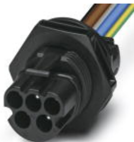
PRC device connector, black, 5-pos., 690 V (IEC 61984), 35 A, crimp connection, 6.0 mm 2 with 150 mm cable length, cut smooth at the end
