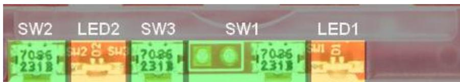
**If you wish to start your Raspberry Pi using the PiJuice SW1 you'll have to connect the micro USB to the PiJuice directly.**
