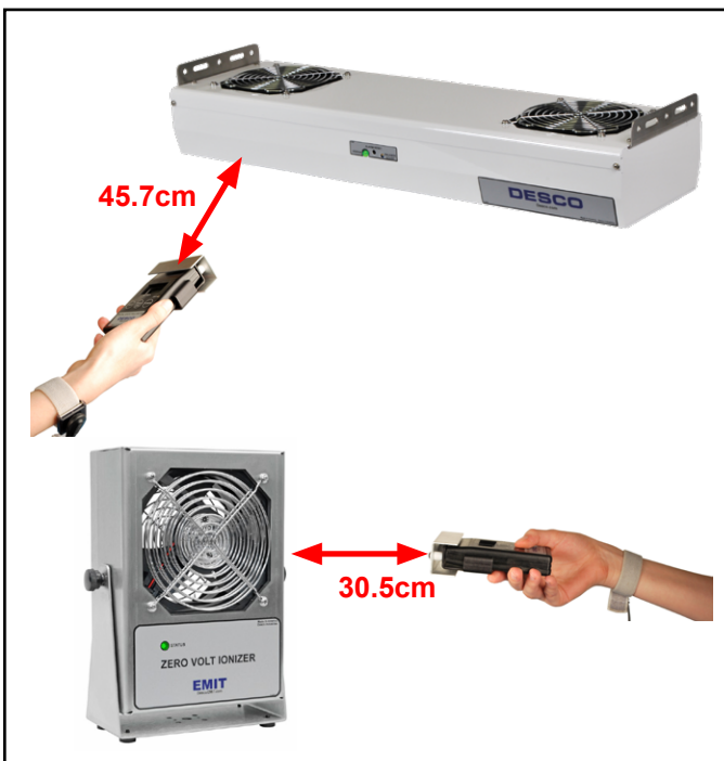
Figure 6. Auditing ionisation equipment with the Digital Static Field Meter and Conductive Plate (Ref: IEC 61340-4-7)
