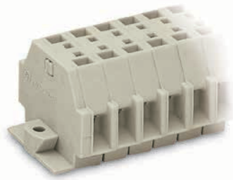
2-conductor Ex e II terminal strip, with mounting flanges, for screw or similar mounting types, 3.2 mm mounting hole diameter, light gray
