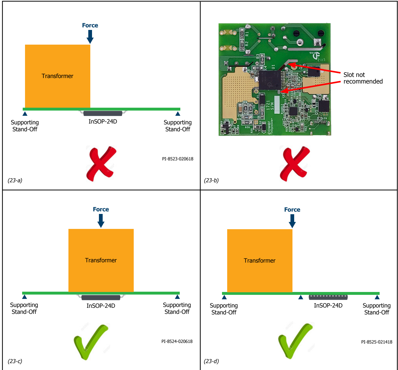
Figure 16. Recommended Position of InSOP-24D Package Shown with Check Mark.
